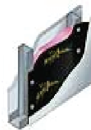
A cutaway rendering of a stud wall layered with a 1/8 inch thickness of sound abatement material and batt insulation beneath the drywall.
